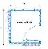
Construction Single Wall External Dimensions 2.2m long x 2.0m wide x 2.5m high Internal Dimensions 2.0m long x 1.8m wide x 2.1m high Total Weight (approx) 1750kg Construction Double Wall External Dimensions 2.9m long x 1.6m wide x 2.7m high Internal Dimensions 2.3m long x 1.0m wide x 2.1m high Total Weight (approx) 2775kg
