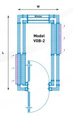
Construction Double Wall External Dimensions 2.6m long x 2.4m wide x 2.7m high Internal Dimensions 2.0m long x 1.8m wide x 2.1m high Total Weight (approx) 3475kg
