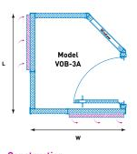
Construction Single Wall External Dimensions 2.1m long x 2.0m wide x 2.5m high Internal Dimensions 1.9m long x 1.8m wide x 2.1m high Total Weight (approx) 1500kg
