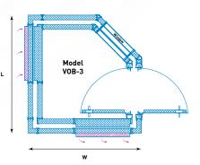
Construction Double Wall External Dimensions 2.5m long x 2.4m wide x 2.7m high Internal Dimensions 1.9m long x 1.8m wide x 2.1m high Total Weight (approx) 2975kg
